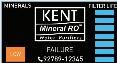
If the TDS level in the purified water is less than permissible range, the indicator would be in Yellow Zone. i.e Low
