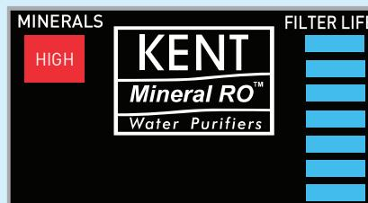
If the TDS level in the purified water is more than permissible range, the indicator would be in Red Zone. i.e High
