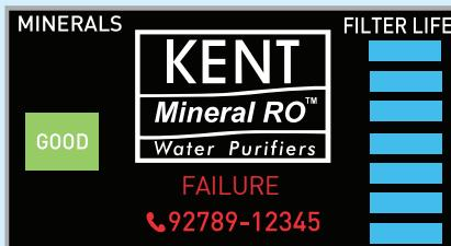
Failure and Call Service Icon will be ON Continuous. Buzzer will beep twice at an interval of 9 Secs for 50 cycles. After 50 cycles buzzer Will go OFF
