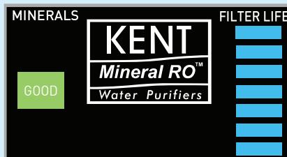
In case of no water input, Kent logo will be Blinking, that means no water input
